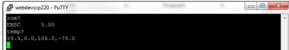
Figure 60: Example of PuTTY command data and response data
