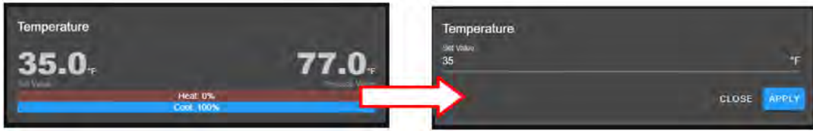
Figure 17.12: Setting new temperature value via the temperature (CTA) pane
