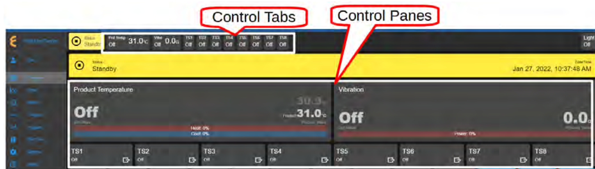
Figure 5.10: Control settings via the control panes
