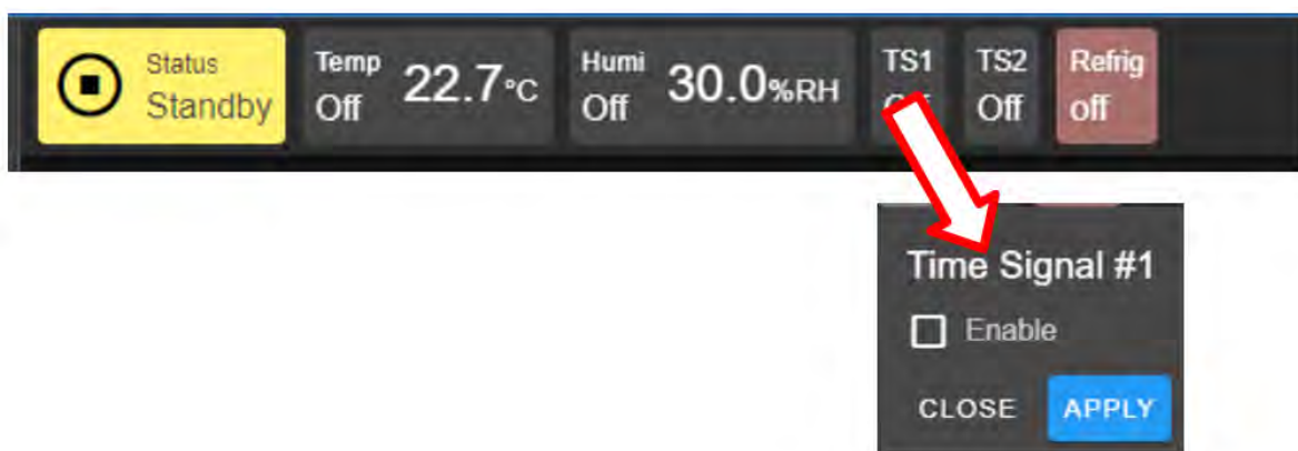
Figure 23.13: Enable or disable time signal setting
