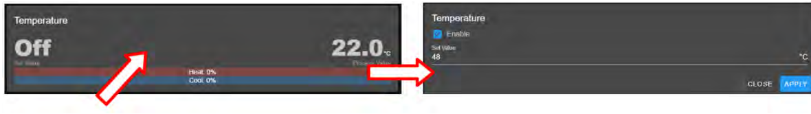
Figure 23.15: Setting new temperature value via the temperature (CTA) pane
