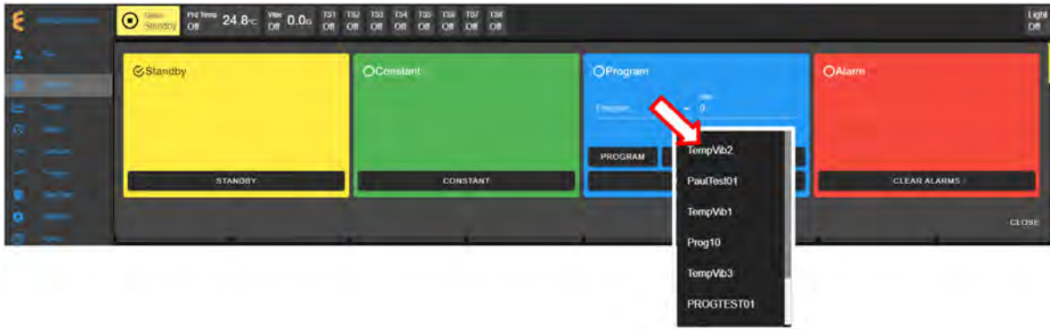
Figure 5.7: Select program to start chamber in Program mode
