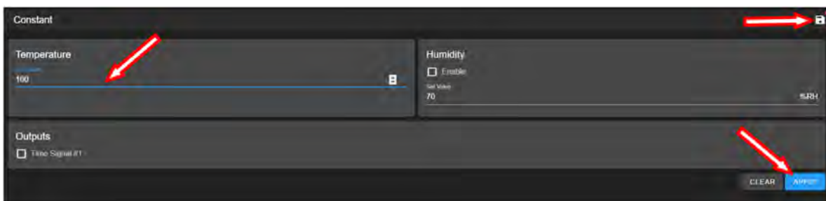
Figure 14.2: Apply new constant setting on temperature
