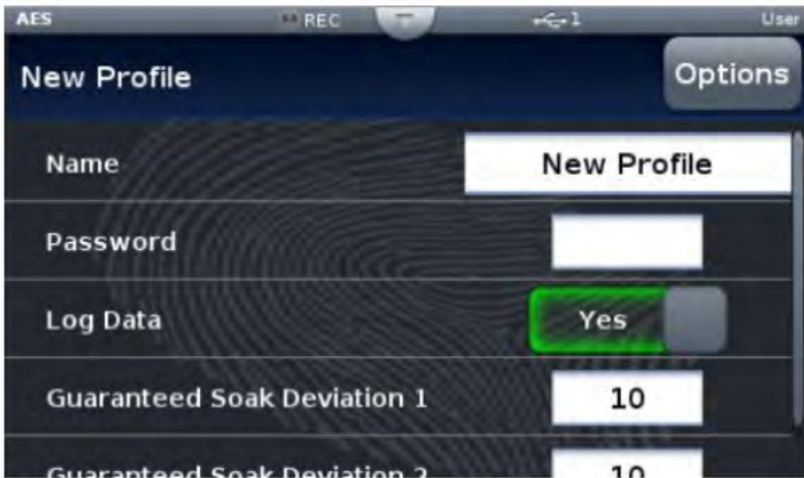
Figure 15.8: F4T with data logging feature
