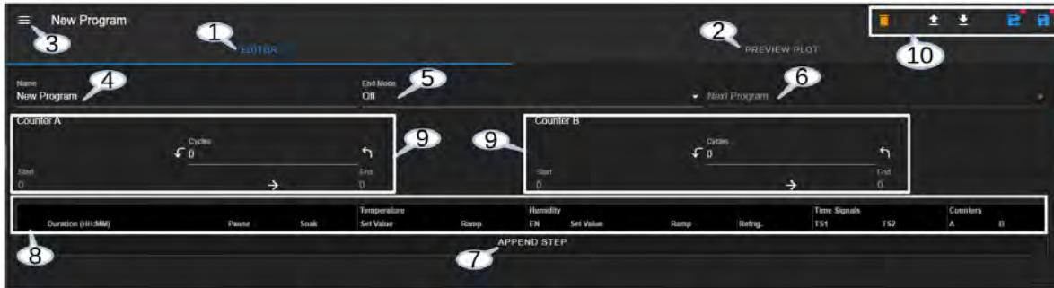
Figure 33.8: The structure and UI of the Programming Editor
