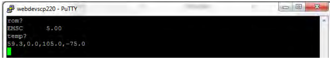
Figure 35.106: Example of PuTTY command data and response data
