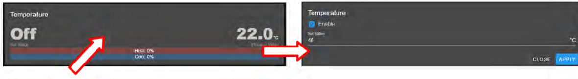
Figure 29.15: Setting new temperature value via the temperature (CTA) pane
