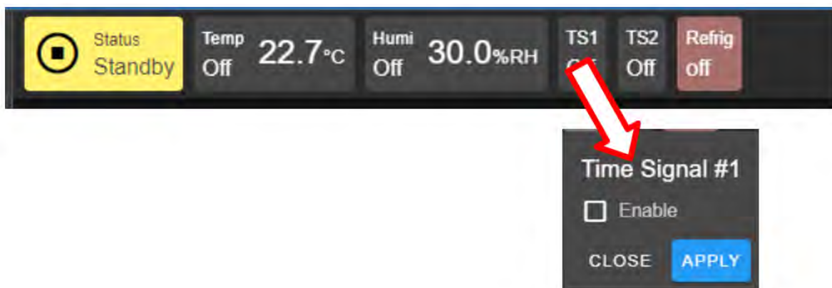
Figure 29.13: Enable or disable time signal setting
