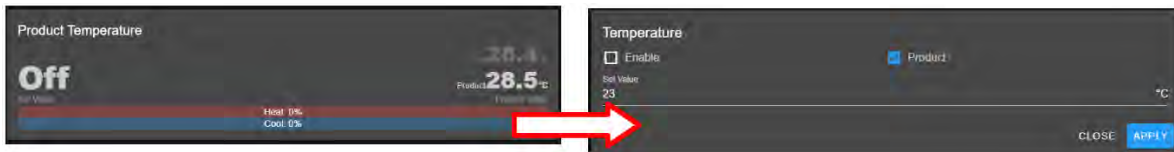
Figure 5.14: Setting new temperature value via the temperature (CTA) pane
