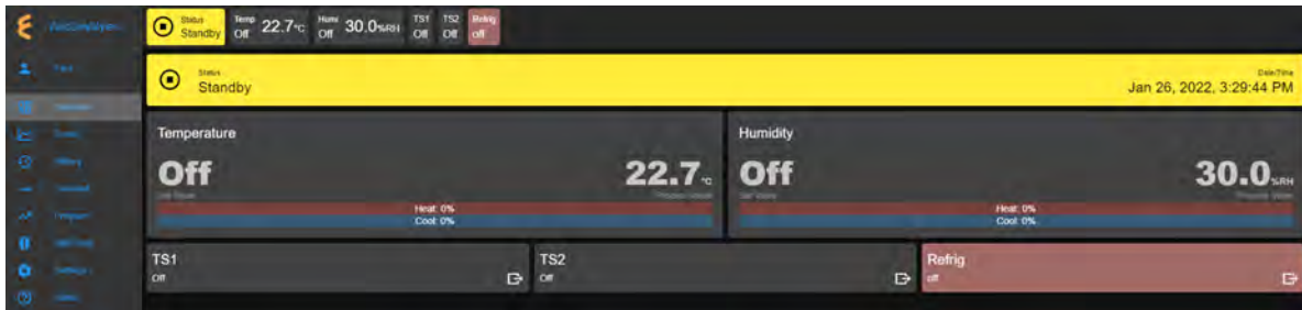
Figure 29.1: Overview page with chamber in Standby mode
