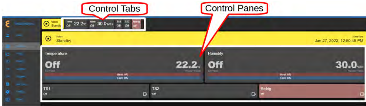
Figure 29.10: Parameter settings via control panes
