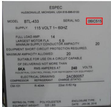
For the serial tag shown to the left the web controller would be accessible at: <http://espec-06ic515/> on windows and <http://espec-06ic515.local> on apple devices or Linux computers.
