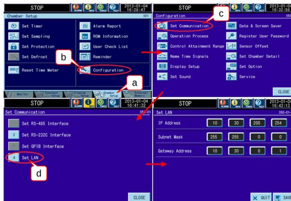
Figure 1.3: EWC IP address on P300 HMI
