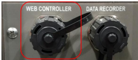
Figure 1.7: Network port on chambers with the following models: EP, EGN, EWP, EWS, EN
