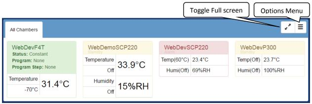
This screen defaults to showing all chambers that it can find that have a web controller with firmware version 2.1.X and newer. If any change are made to the layout and saved then the page will load the saved configuration instead.
