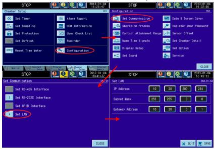
b. The IP address can be found via the "Espec Web Controller Locator" utility included on the web controller and or chambers manual CD. The utility will scan look for web controllers version 2.0.0 and higher immediately after opening it, the IP Addresses are listed in the second column. Clicking on the IP address will open that controller via its IP address, the host name will be clickable if the computer can resolve it.
