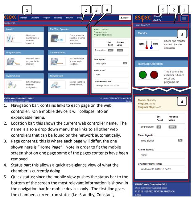
Program, Alarm) and the second line the conditions inside the chamber i.e. temperature and
